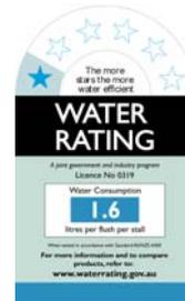
Water rating when used with cistern. (Tested with Caroma Water Wafer 600mm flush pipe)
