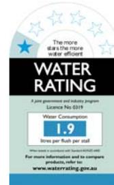
Water rating when used with automatic flushing device. (Tested with Reece Sensor Flush 1000mm flush pipe)
